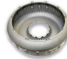
Combustion chamber made in one piece by SLM : dilution holes and multi-perforation . Inconel 718 metal (EADS IW)
