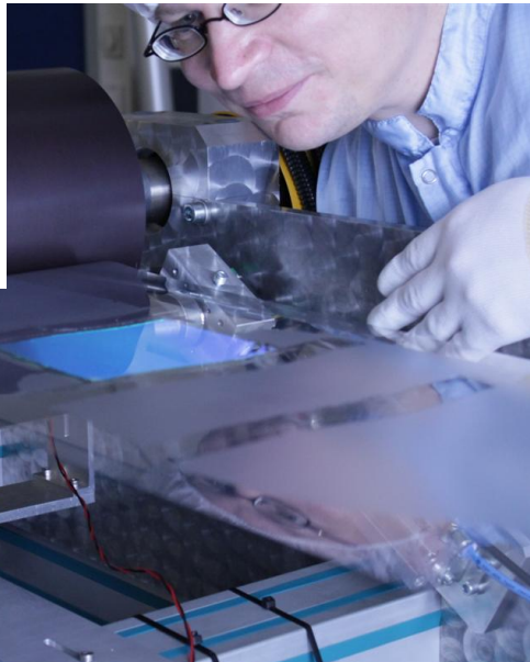
R2R embossing of out-couple structures for OLED stacks
